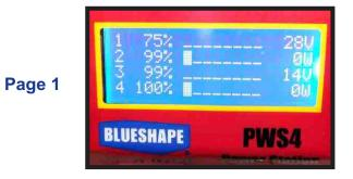
For each installed battery, the state of charge is shown in percentage.
